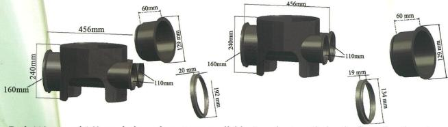
Both 110mm and 160mm drainage layouts are available. In order to optimize the flow directions, branch inlets are provided as well. Inspection chambers come can be joined to uPVC (160mm/110mm). The chamber base has 2 110mm inlets (90 degree to the central channel). Push fit joining using rubber rings is done between the uPVC pipes and the Inspection Chamber.
