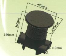
The MOVA Inspection Chambers are manufactured and tested to BS EN 13598-1:2010. They are suitable for use in underground drainage and sewerage system to a maximum depth of 1.25m.
