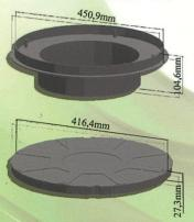
The inspection chamber frame and cover is made of high impact and UV-stabilizer ABS. The frame fits into the inner or the riser and is sealed by a water tight rubber seal. The matt finished cover (for anti slip) is screwed down in the frame for security and reduced risk of unwanted removal. MOVA chamber frame & cover have been tested to BS EN 1253-4 for water tightness, odour tightness and backflow tightness.
