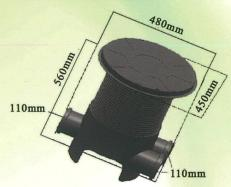
The MOVA Inspection Chambers are simple push-fit assembly. It requires considerably less labour and more economical than the traditional brick or reinforced concrete construction. MOVA Inspection Chamber allows for 2 inlet pipes and one outlet pipe. Extra inlet pipes can be fabricated according to site requirement.
